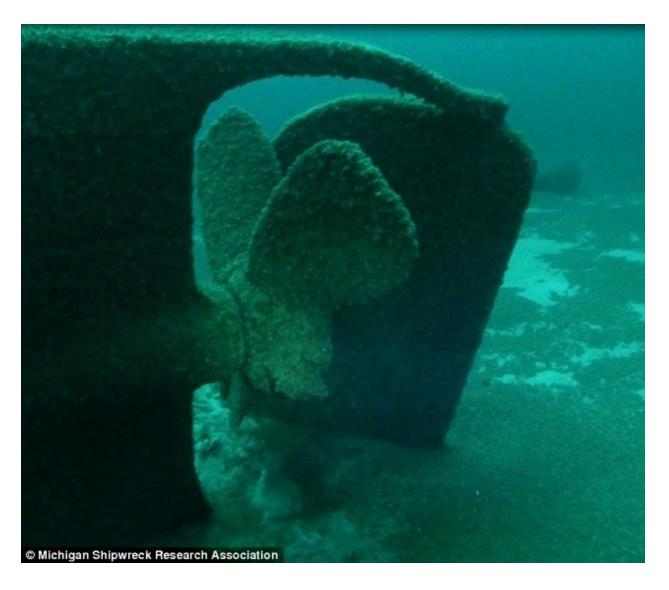
The Michigan Shipwreck Research Association (MSRA) captured the first-ever footage of the SS William B. Davock shipwreck, determining a rudder the broke in the storm struck the propeller (pictured)
