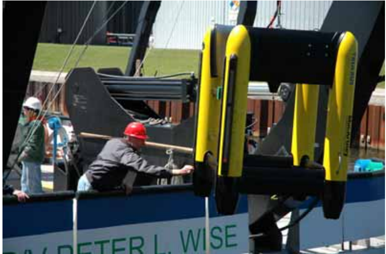
Deployment of towed sensor array on U.S. EPA research vessel. Photo: U.S. EPA Great Lakes National Program Office.
